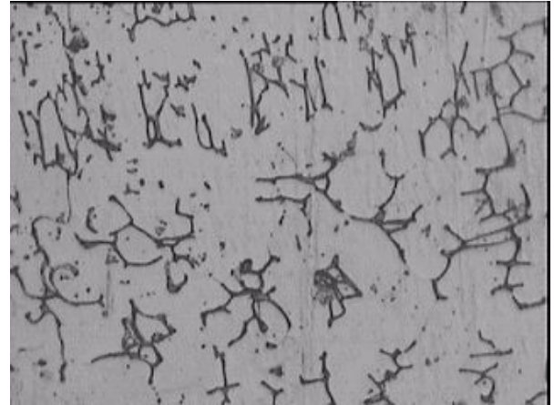
Fig. 3a : Bulk weld metal, 1 mm from the clad interface Etchant : Aquaregia. Taper section, 400X
