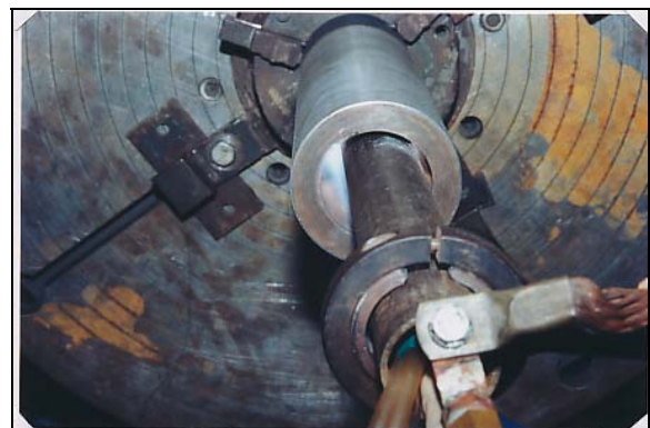
Fig. 18: Hardfacing of grid plate sleeve (inner diameter about 80 mm) using an indigenously designed PTAW torch
