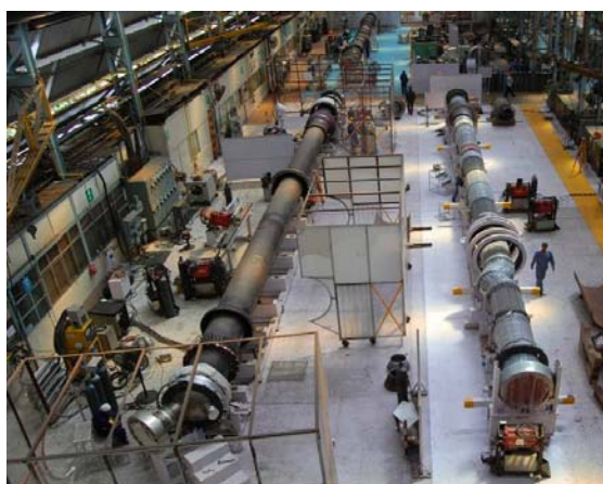
Fig. 5: Steam generators under fabrication
