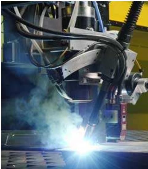
Fig 5 : HLAW Welding in operation
