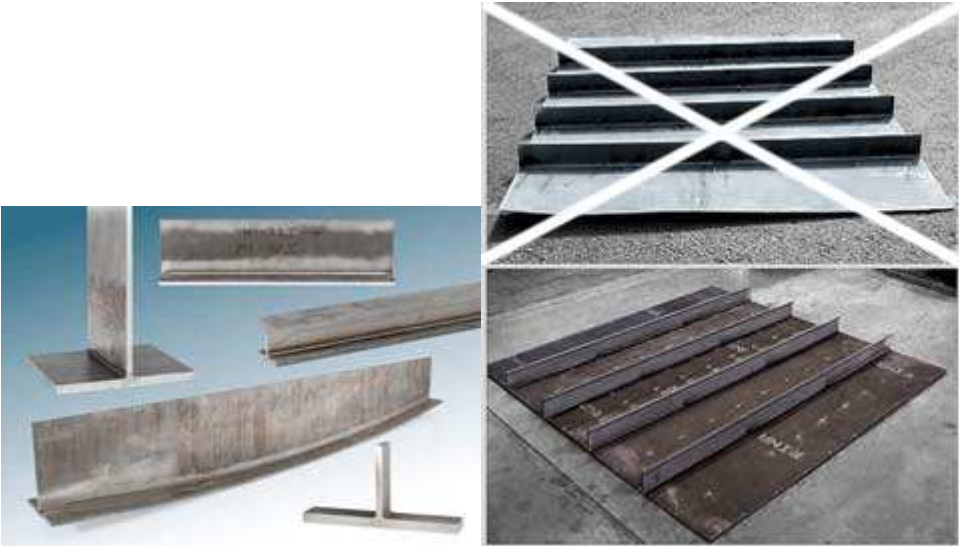
Fig 6 : Parts welded with HLAW vs those conventionally welded
