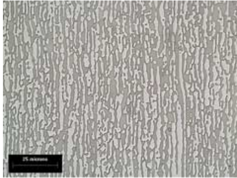
Fig 3: Duplex Stainless – HLAW weld microstructure
